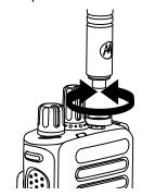
**2** To remove the antenna, turn the antenna counterclockwise.
