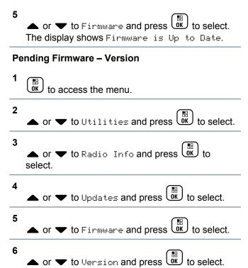
If there is a pending Option Board firmware file, the display shows the pending firmware version
