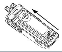
2 To remove the battery, turn the radio off. Move the battery latch (A) into unlock position and hold, and slide the battery down and off the rails.
