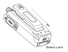
To remove the battery, turn the radio off. Move the battery latch into unlock position and hold, and slide the battery down and off the rails.
