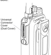
Place the universal connector cover loop over the attached antenna. Slide it all the way down to the base of the antenna.
