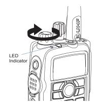
NOTE: The Home screen does not light up during a power up if the LED indicator is disabled (see *Turning the LED Indicator On or Off* on page 95).
